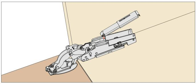
Lift the flap slightly and clip the other end of the Smove into position. This operation is tool free.
